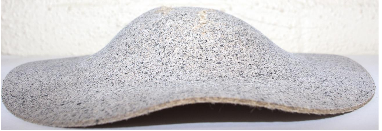
Figure 6.6: Buckling of a flax/pp composite tested at 120°C.
